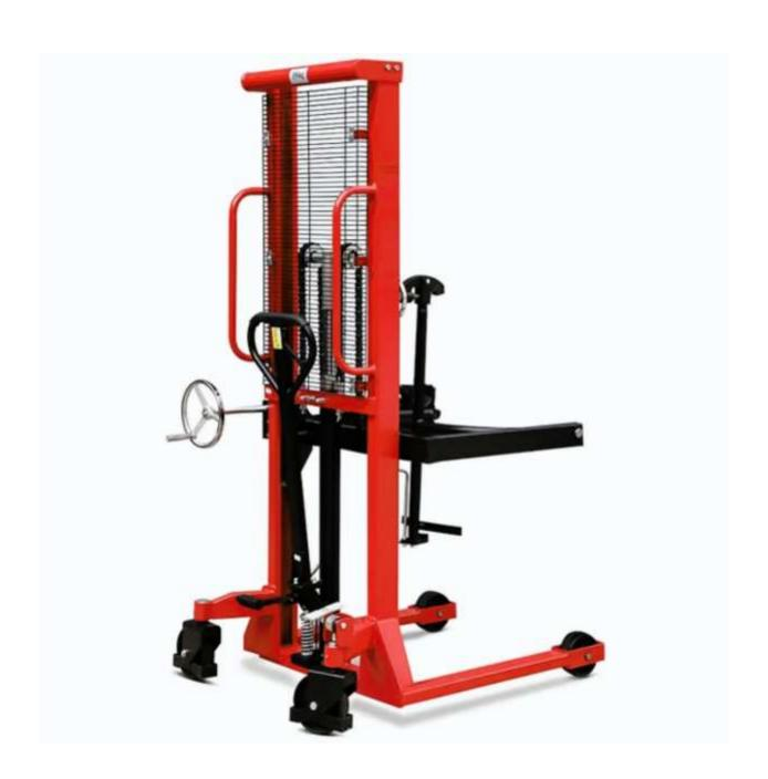
\* The eagle clip on the drum truck is forged by high quality steel plate, the chuck can be tightened through move the steering by your hand, which can fix the oil drum quickly and firmly without falling off.
